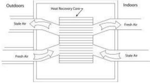
One way to minimize air quality and moisture problems in a home, without opening a window, is by the installation of a mechanical ventilation system such as an air-to-air heat exchanger. An air-to-air heat exchanger brings two air streams of different temperatures into thermal contact, transferring heat from the exhausting inside air to incoming outside air during the heating season.
